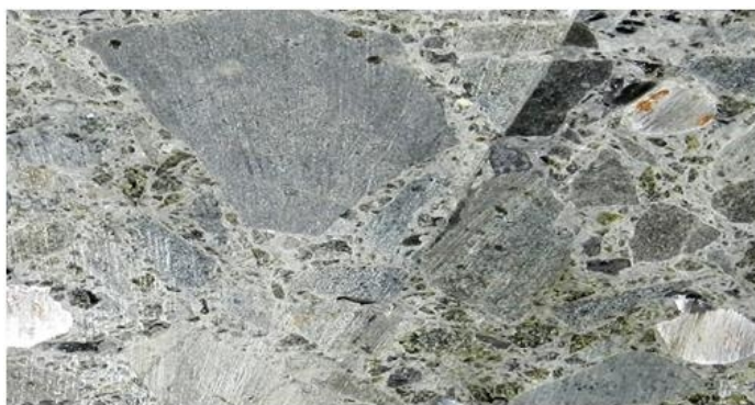
Plate 4 Microscopic arrangement of BFS made concrete
