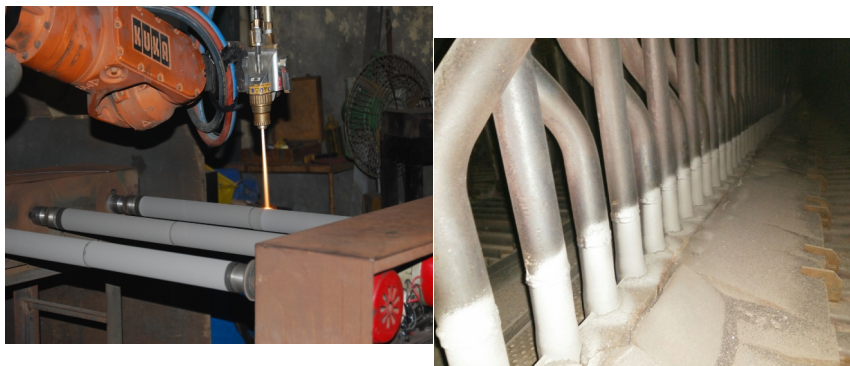
Fig 1 WC-300 HVOF Coating at 125 0 C for coating thickness 500 \mu m
