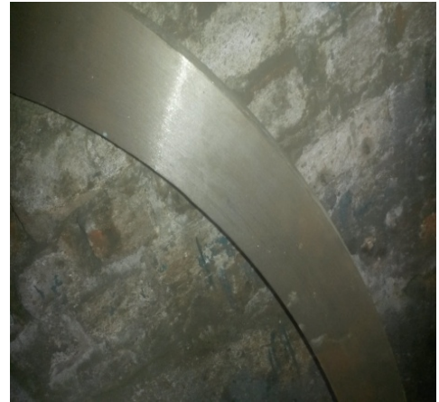
Fig.9 closed view of Machined Surface (part free from shrinkage porosity)
