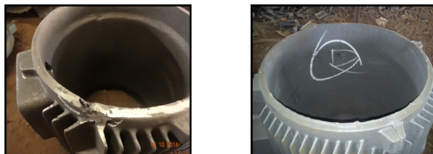
Fig.2 Sand inclusion defect in actual Motor Body Casting
