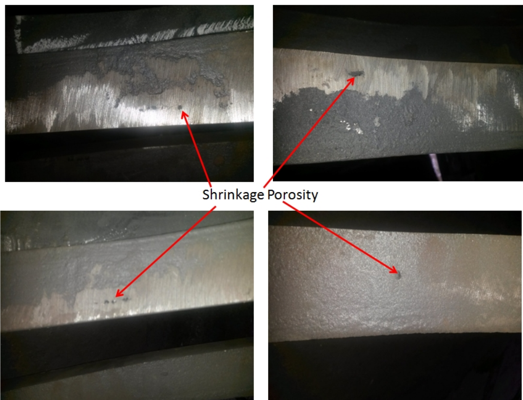
Fig. 2: Shrinkage porosity observed inside the casting at different locations
