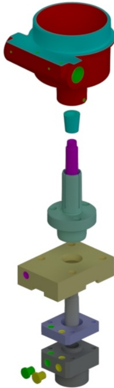
Fig. 10. Exploded Collet-Assembly with Hydraulic cylinder
