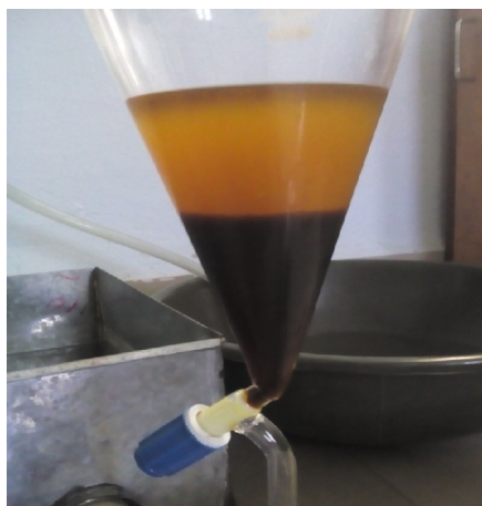
Fig-2 separation of glycerol and impurities and KOME
