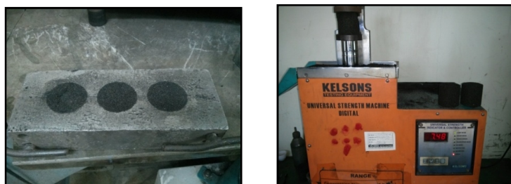
Fig.7 Compressive strength test with help of UTM
