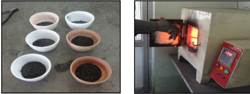
Fig.4 LOI test performed at Industry
