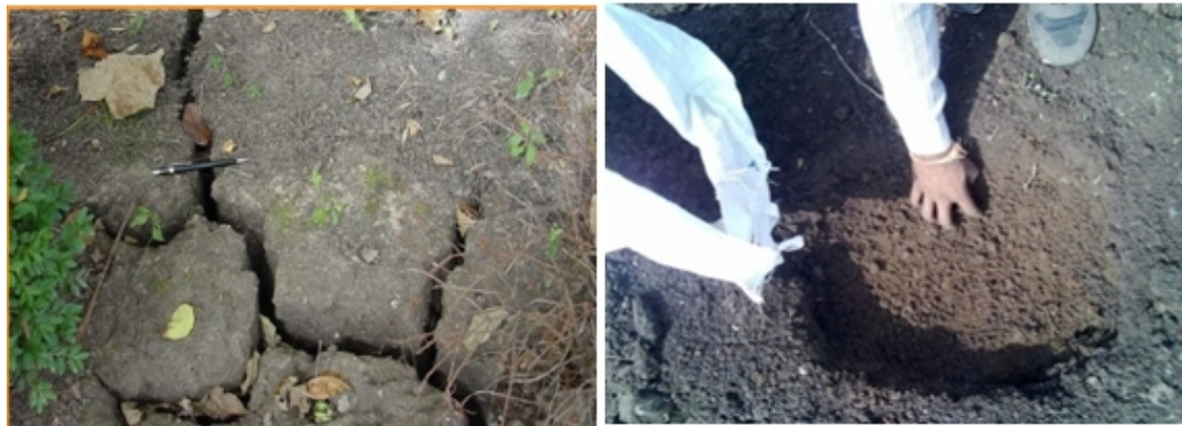
“Fig. 1.(a) Behaviour of Black Cotton Soil (b) Sample Collection of Black Cotton Soil”
